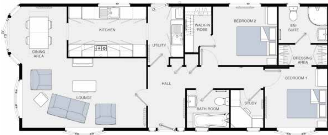
50' x 20' (15.240m x 6.012m) 'L' shaped lounge / dining area, kitchen, utility room, study, 2 bedrooms (master with en-suite and bedroom 2 with walk-in wardrobe) and family bathroom
